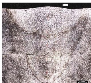
Figure 10: Example of penetration depth measure
