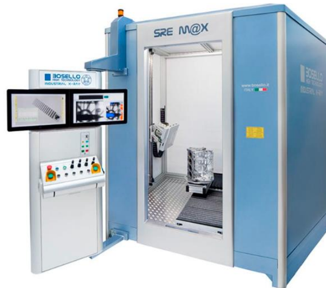
Figure 5. Digital radiographic control system.
